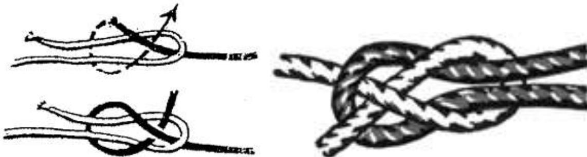
The sheet bend is the most important knot for joining two rope ends, especially if the ropes are of different sizes. Sailors named it in the days of sailing ships when they would "bend" (tie) the "sheets"(ropes attached to the clew of the sail).
