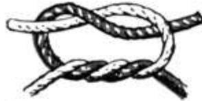
The surgeon's knot is a simple modification to the square knot. It adds an extra twist when tying the first throw, forming a double overhand knot, thus adding friction which makes the knot more secure. This knot is named for the fact that it is commonly used by surgeons in situations where it is important to maintain tension on a suture. Surgeon's knots are used in fly fishing as well as in tying packages.
