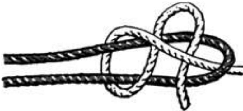
The slippery sheet bend is simply an ordinary sheet bend with a bight left in the smaller rope. This bight makes it "slippery" because it can be untied quickly, merely by a tug on the free end of the rope. It is a valuable knot for use when you expect to tie and untie it often.
