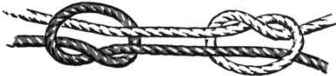
The Fisherman's knot is a specialized bend. It consists of two overhand knots wrapped around each other. It requires little dexterity to tie, so is often used in stubborn materials. When tightened, it becomes fairly compact, and the free ends can be cropped very close to the knot. These qualities make it very useful for fishing line--it is less likely to jam a fishing rod, and is easier to tie with cold, wet hands.
