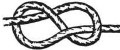
The figure-eight knot is very important in both sailing and rock climbing as a method of stopping ropes from running out of retaining devices.
